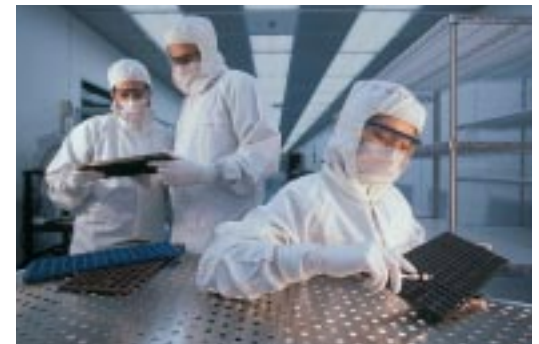
After final manufacturing, packaged ICs are transported to makers of electronic goods in Entegris' JEDEC trays to ensure the best protection.
