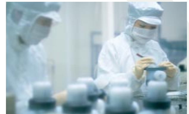
In Japan, workers assemble valves destined to protect the ultrapure and corrosive chemicals used to manufacture ICs.
